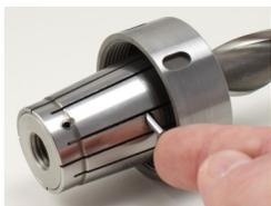
Insert Pin into the Pin Hole
