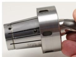
Once the pin is fully inserted pull out on the cutting tool so the back of the flat is tight against the pin
