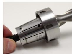
Insert the preset screw finger tight against the back of the cutting tool to hold the cutter in place and eliminate gap and movement
