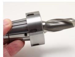
Fully insert cutter into the collet
